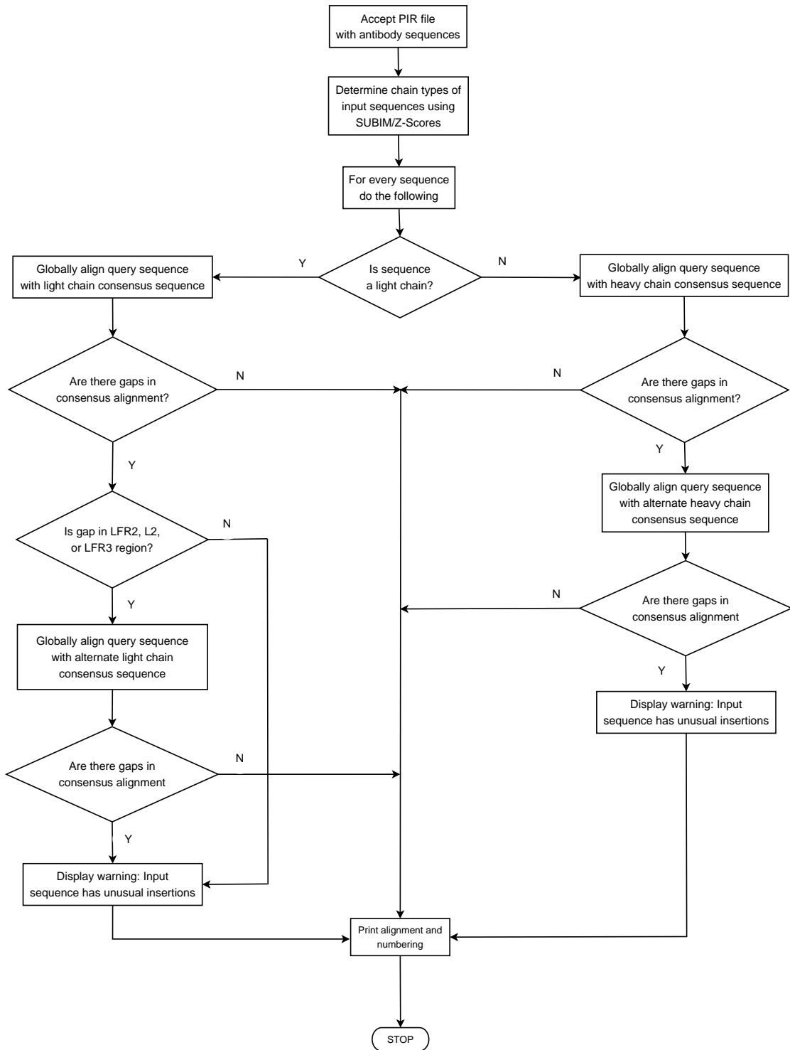
Figure 4.7: Overall algorithm for the alignment-based numbering method.
